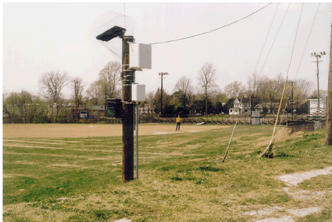
Figure 4. TDR data acquisition system. Cable tester, data logger and modem are in the upper enclosure; multiplexer is in the lower enclosure; system is powered by a deep cycle battery that is trickle-charged by the solar panel.
